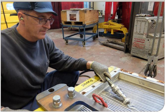
With over 30,000 units in tough process duties around the world, Alfa Laval Compabloc has a well-earned reputation for robust and efficient thermal performance. Although Compabloc's design requires little service or cleaning, periodic examination of the unit's condition helps you maintain the highest level of mechanical integrity and operating performance to maximize both uptime and the lifespan of the unit.
