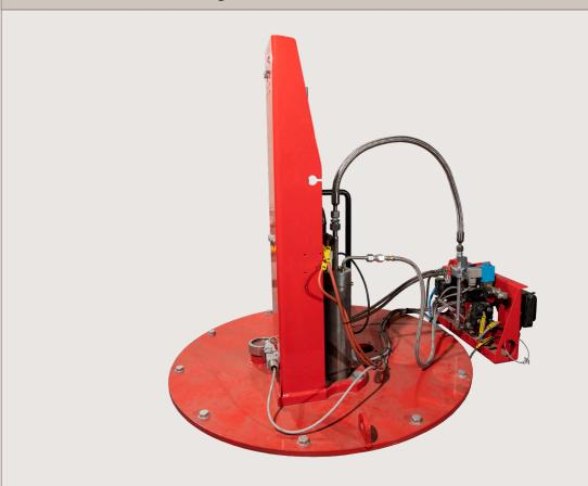
The flexible fuel oil hose modification kit contains everything needed for vertical mounting of the flexible fuel oil hose on your Alfa Laval Aalborg KBSD/A burner. Mounting in a vertical position will decrease the tension placed on the hose when the lance is in movement.
