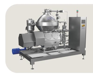
The system can be selected with an optional ProCarb<sup>TM</sup> feature - a patented inline carbonation technology that boosts productivity by combining rapid clarification with carbonation. This combination reduces the processing time from crash cooling tanks to packaging from 3 days to 3 hours.
