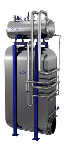
The Aalborg AV-6N is a robust, highly efficient water tube boiler for utilizing heat energy from engine/gas turbine exhaust or process industry flue gas that would otherwise be released into the air. This means reduced fuel use, leading to remarkable cost savings and lower CO<sub>2</sub> emissions.
