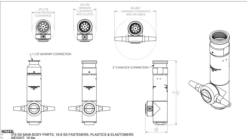
INLET: 1-1/2" SANITARY INLET, 1-1/2" SLIP FIT & 2" CAMLOCK ADAPTER/1-1/2" FNPT
