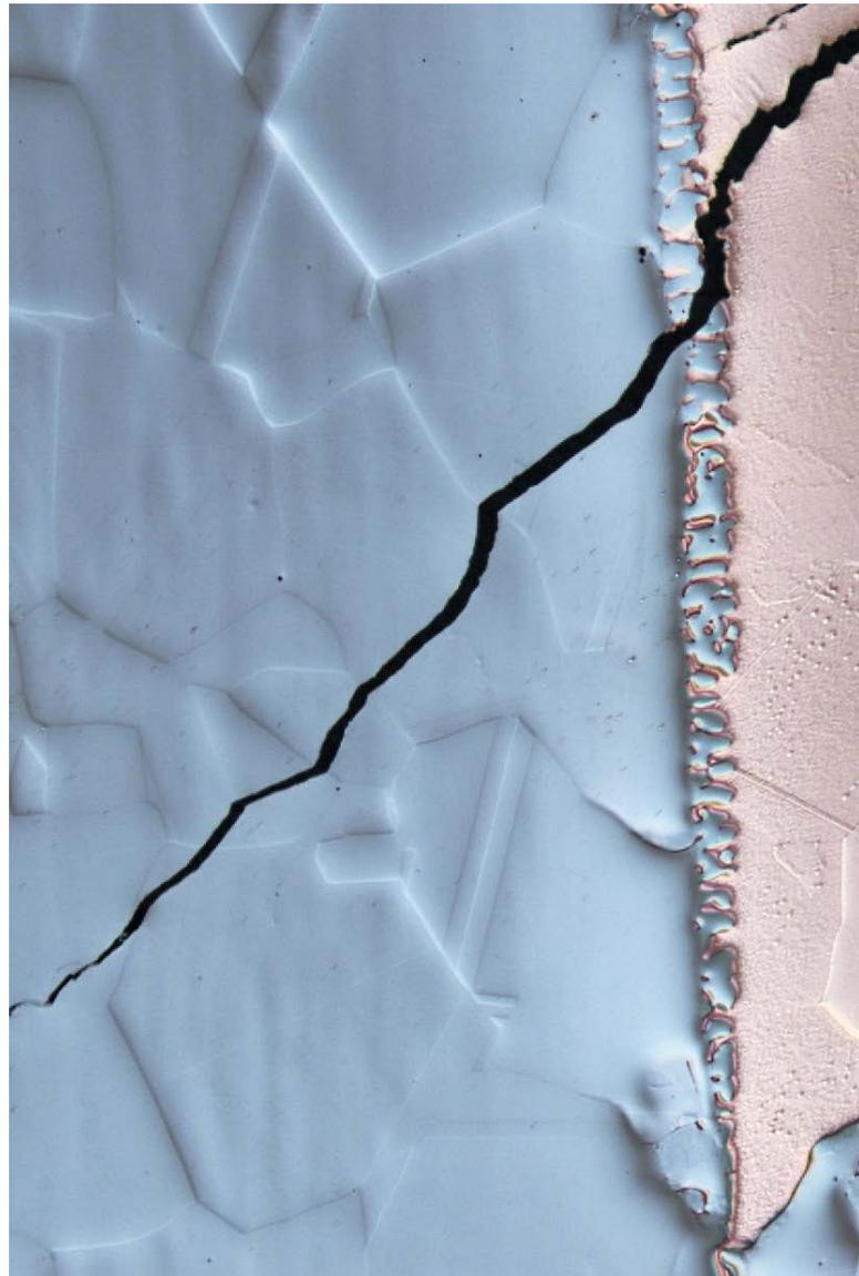
*Fatigue is a phenomenon that occurs due to fluctuating tensile stress caused by vibrations or pulsating pressures. A failure investigation can confirm fatigue based on the characteristics of the crack.*
