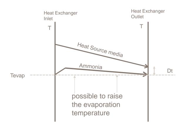
In general it is possible to obtain 2K closer approach than with other heat exchanger technologies at comparable size and cost
