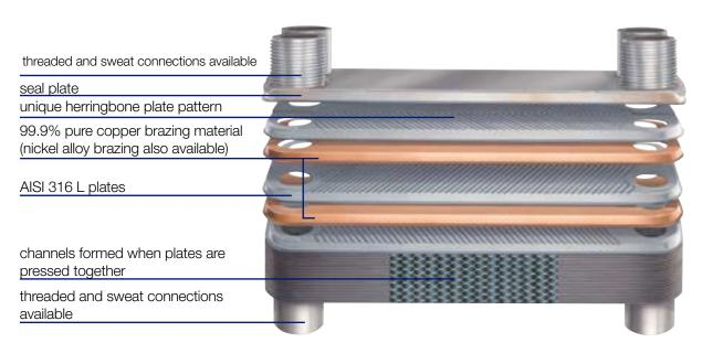
The brazed plate heat exchanger is the most compact heat exchanger on the market today. Its high heat transfer efficiency in combination with its compact design equals a compact heat exchanger for a wide range of heating, cooling, evaporating and condensing duties.
