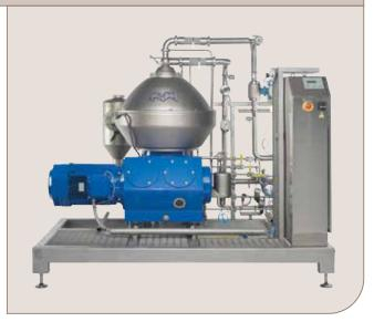
It has a clarifier type of bowl with a conventional top-fed design. The liquid outlet is sealed by the Oxystop hydrohermetic seal that prevents oxidation of the clarified product. The separator has variable discharge volume, which leads to minimum product loss.
