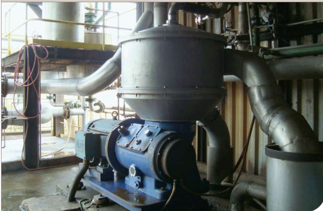
One of the two upgraded Alfa Laval separators. Together, in terms of capacity, they are the equivalent of a third machine.
