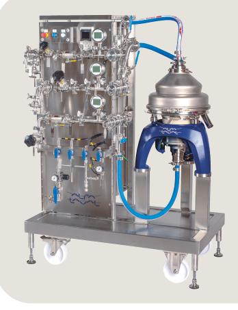
design. The machine can be configured for different separation duties, different disc angles and different solid/ heavy phase removal by different conversion kits. The Alfa Laval Explorer can be configured for two-phase separation as well as three-phase separation, with solids removal by discharge or using the Alfa Laval TopStream technology for continuous solids/heavy phase removal.
