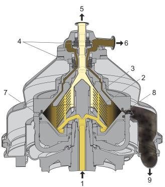
Typical bowl drawing for a solids-ejecting separator. The details illustrated do not necessarily correspond to the separator described.
