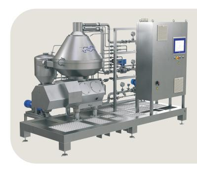
All metallic parts in connection with the process liquid are made of stainless steel.
