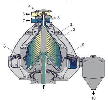
Typical bowl drawing. The details illustrated do not necessarily correspond to the separator described.
