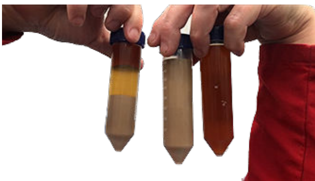
Example: Salmon process. From left feed, de-oiled slurry, and clean oil.
