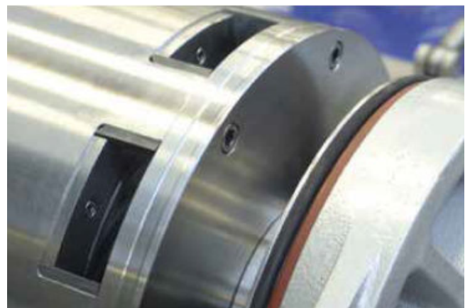
Fig 2. 360° solids discharge, free from blocking
