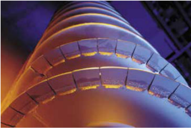
Fig 4. Sintered tungsten carbide tiles as wear protection for conveyor flights
