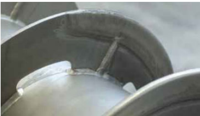
Fig 5. Flame sprayed tungsten carbide wear protection on conveyor flights
