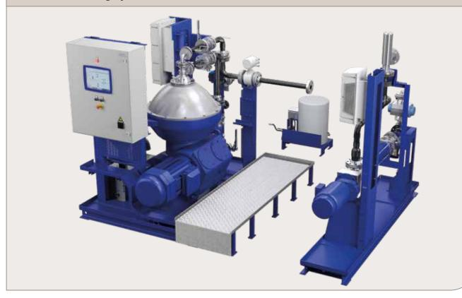
PureScrub H2O uses high-speed centrifugal separation to clean scrubber wash water in compliance with IMO legislation. It is the advanced water cleaning unit (WCU) used in closed-loop or hybrid configurations of the Alfa Laval PureSOx exhaust gas cleaning system, but it is also sold as a standalone product for use in wet scrubbers not designed by Alfa Laval.
