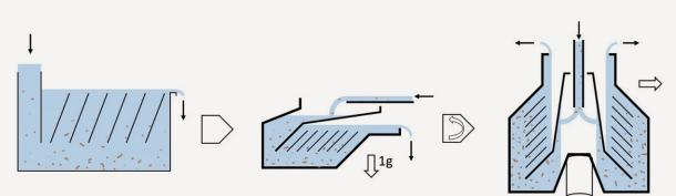
From sedimentation tank to centrifugal separator
