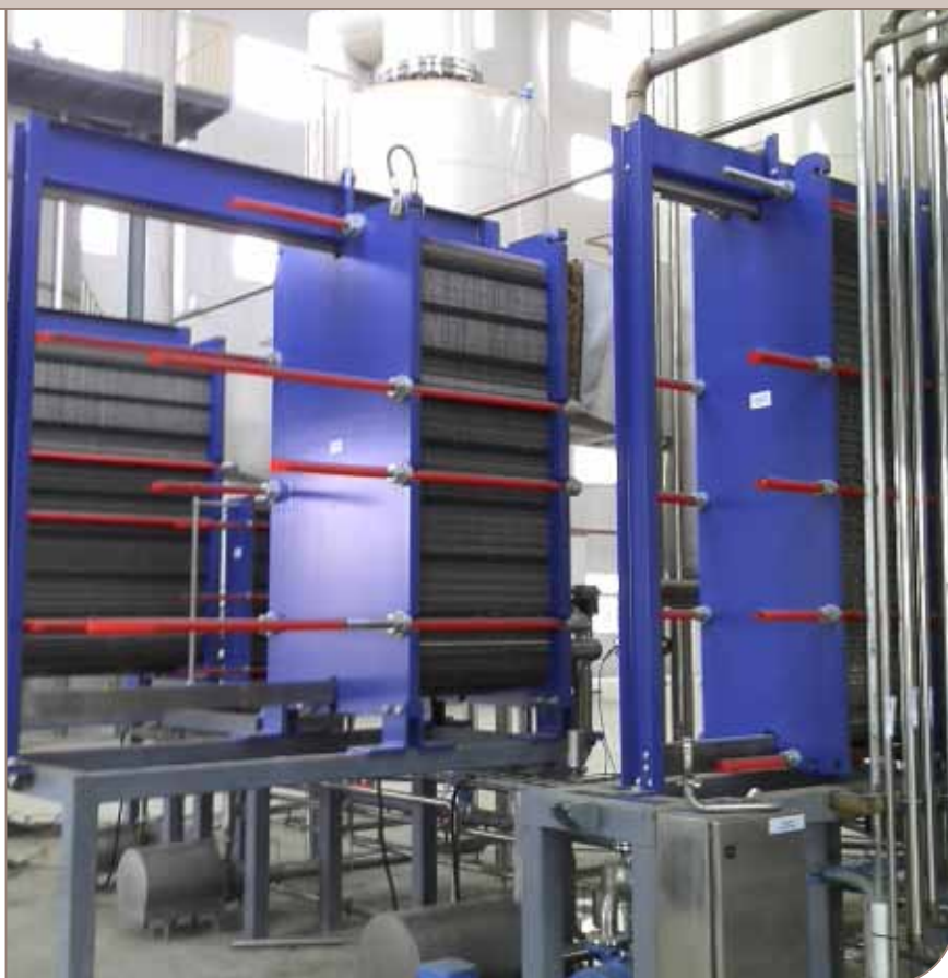
Two AlfaVap 500 evaporators and an AlfaCond 400 condenser installed at the Biok plant.
