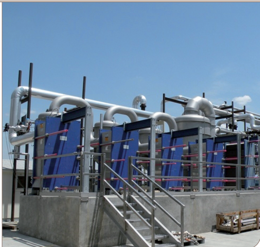
Multi-effect AlfaVap evaporation system for grape must
