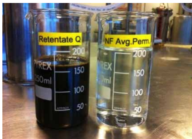
Effective colour removal – samples showing NF retentate (10x concentrated colour) and average NF permeate (purified NaCl solution) for reuse.
