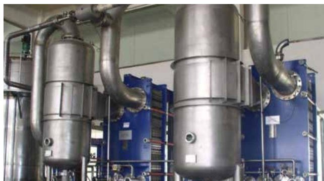
AlfaVap evaporator system, featuring fully automatic operation with no manpower requirements.
