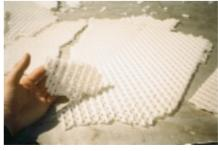
The illustrations shown above are from a plant which was deliberately scaled up with calcium sulphate in order to successfully test and prove 100% cleanability.
