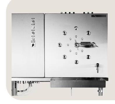
The sampling panel, which is mounted on adjustable legs, is connected via pipes of Ø10 mm to the pneumatic sample valves on the tanks. The connections can either be stainless steel pipes or Teflon hoses, with or without insulation, depending on local conditions. As can be seen from flow sketch, the pipe work creates a ring main between the sampling panel and the sample valve.
