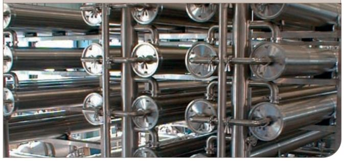
The Alfa Laval Membrane RO/NF system is a cross-flow reverse osmosis (RO) and nanofiltration (NF) membrane system designed for automatically controlled continuous product concentration and water recovery.
