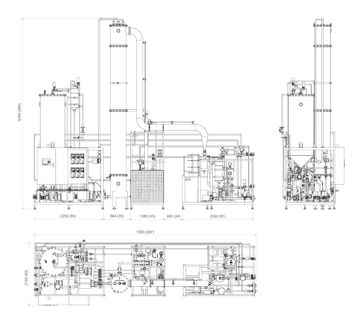
The Alfa Laval De-alcoholization module is fully assembled and dimensioned as shown above, as example, for the 10 hl/h case. Dimensions are indicative in mm (inches).
