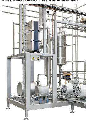
The De-alcoholization module's condensate cooling section.
