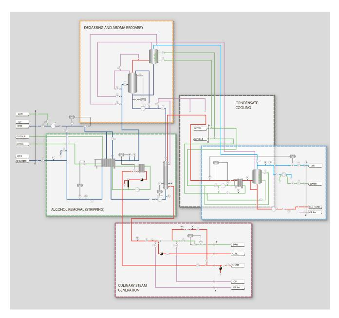
Flowchart for the De-alcoholization module, featuring the major process sections: alcohol removal, degassing and aroma recovery, culinary steam generation and condensate cooling.
