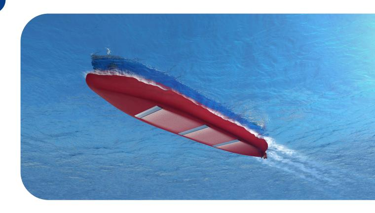
Alfa Laval OceanGlide is an easily installed air lubrication solution with fluidic technology. By creating an even and controllable air layer across the entire flat bottom of the vessel, it provides the best possible setup for drag reduction. This improves energy efficiency and reduces fuel consumption, which results in lower fuel costs and CO<sub>2</sub> emissions.
