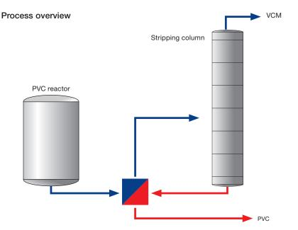
The PVC slurry interchanger recovers heat from the stripping column and uses it to preheat the feed. Exchanging the existing shell-and-tubes for two Alfa Laval spiral heat exchangers resulted in dramatically reduced maintenance needs and increased production capacity. As an added bonus the new heat exchangers recover more heat, leading to annual steam savings of 110,000 euros.
