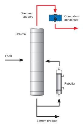
Using four Alfa Laval Compablocs as overhead condensers, the company now recovers a total of 23.6 MW of heat, resulting in energy savings of roughly 2.7 million euros annually.
