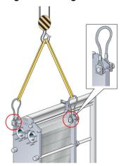
Figure 7: Lifting Semi-welded TK20 and Semi-welded T20.
