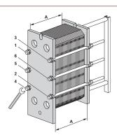
For manual tightening, the tightening torque has to be estimated.
