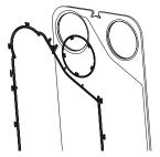
6 Repeat the procedure until all plates that are needed to be regasketed are done. Close the heat exchanger according to *Closing* on page 38.
