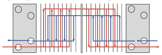
Figure 3: Example of a multi-pass set up.
