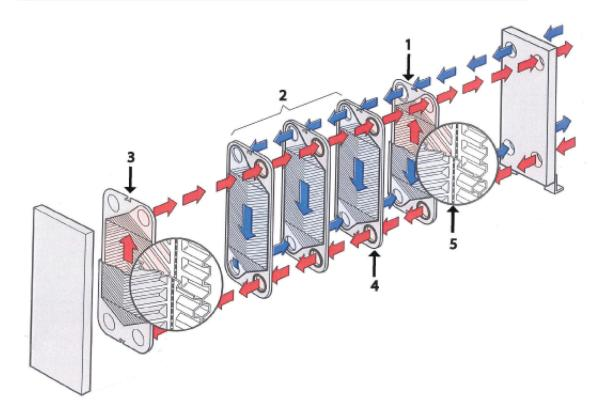
Figure 2: Example of a single-pass set up.
