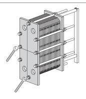
(10) Use the tightening bolts to open the heat exchanger. During the opening procedure, keep the frame plate and pressure plate parallel. Skewing of the pressure plate during opening must not exceed 10 mm (2 turns per bolt) across the width and 25 mm (5 turns per bolt) vertically.
