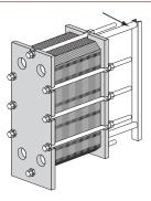
7) Mark the plate assembly on the outside by a diagonal line.
