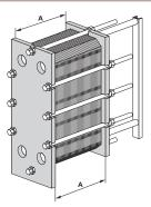
Loosen and remove the locking bolts. Identify them according to **Bolt configuration** on page 34.
