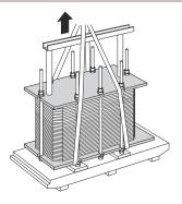
Place the heat exchanger on the timber beams.
