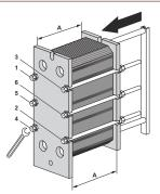
7 Tighten the four bolts (1), (2), (3), (4) or the six bolts (1), (2), (3), (4), (5), (6) evenly until dimension **A** has been reached.
