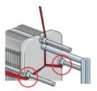
Figure 6: Lifting TS6.
