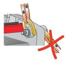
Figure 7: Lifting device for AQ20S. Use the four inner eyes when lifting the heat exchanger. Do NOT use the transport securing points! Securing equipment is needed.
