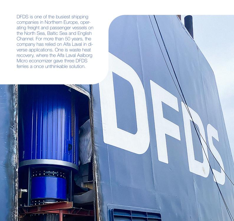
In an Aalborg Micro, you have only around 200 kilos of water ... That makes the Micro very, very light and compact compared to conventional systems.
