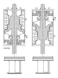
Pneumatic movement upwards
