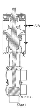
The plug opening for different change-over valves and actuator size is shown below.
