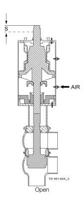
The plug opening for different change-over valves and actuator size is shown below.
