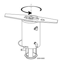
Rotate cylinder with service tool!
