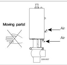
To avoid water hammering, it is recommended to install the valve so that the flow is against the spring closing direction.
