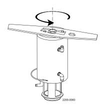
Rotate cylinder with service tool!
