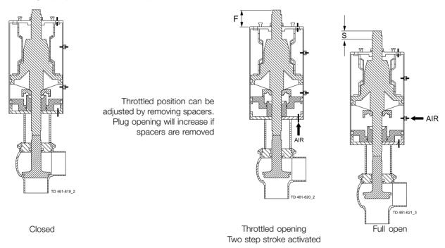
The plug opening for different shut-off valves and actuator size is shown below.
