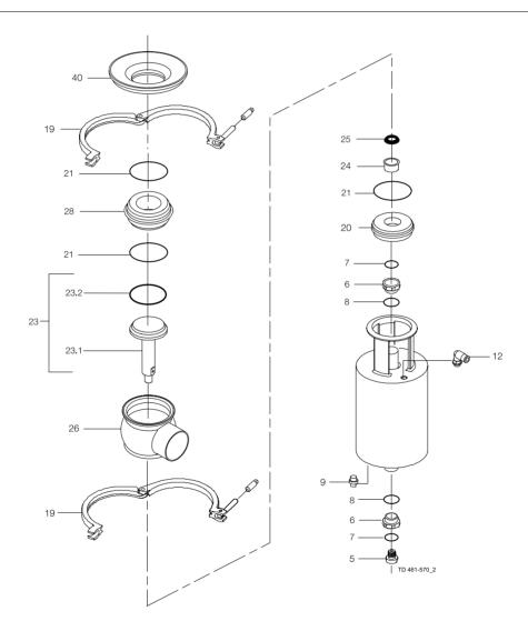
The drawing shows Unique Single Seat Valve - Tank Outlet. The items refer to the parts list in the following sections.
