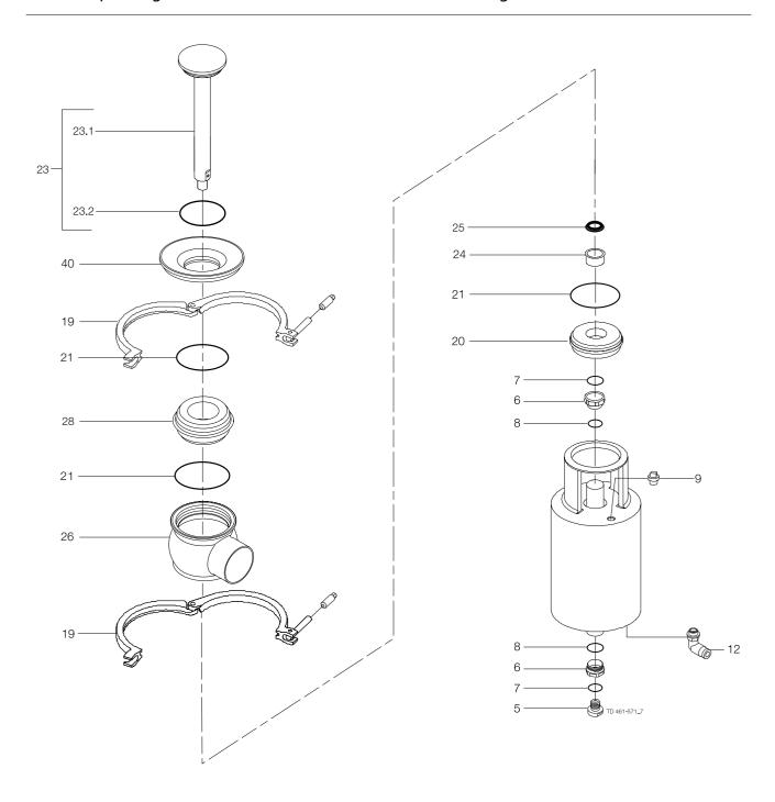
The drawing shows Unique Single Seat Valve - Tank Outlet - Reverse Acting. The items refer to the parts lists in the following sections
