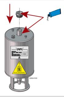
Fit the aligning spindle to the actuator spindle, and then mount the socket wrench.
