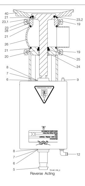
The drawing shows Unique Single Seat Valve - Tank Outlet - Reverse Acting. The items refer to the parts lists in the following sections
