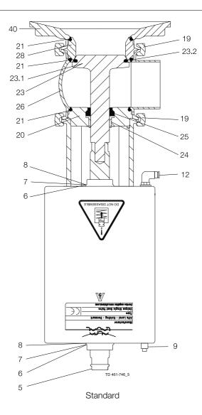
The drawing shows Unique Single Seat Valve - Tank Outlet. The items refer to the parts list in the following sections.
