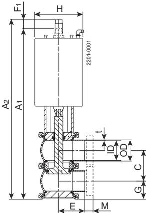
Figure 1. Shut-off valve
