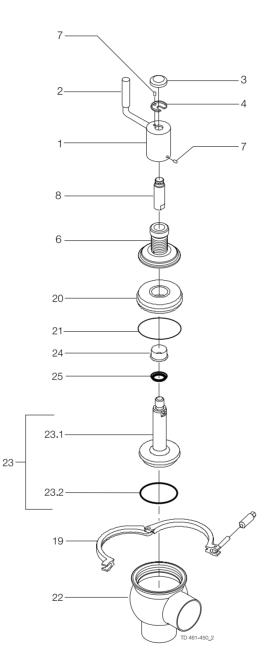
The drawing shows Unique Single Seat Valve - Manual operated, Shut-off. The items refer to the parts lists in the following sections
