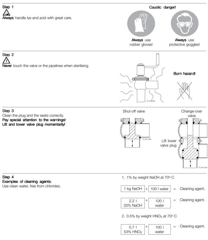
The valve is designed for cleaning in place (CIP). Study the instructions carefully and pay special attention to the warnings! NaOH = Caustic Soda.  $HNO_3 = Nitric acid.$
