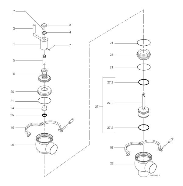
The drawing shows Unique Single Seat Valve - Manual operated, Change-over. The items refer to the parts lists in the following sections
