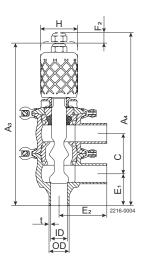
Figure 4. Manual change-over valve
