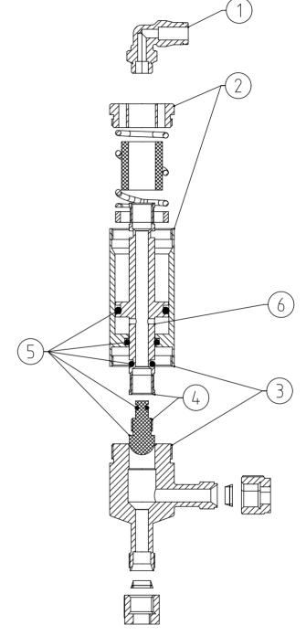
Maintain the valve regularly. Study the instructions carefully and pay special attention to the warnings! Always keep spare rubber and seal parts in stock. Check the valve for smooth operation after service.
