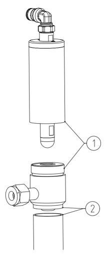
The valve can be mounted in any position. However, care must be taken to facilitate complete drainage from the valve.
