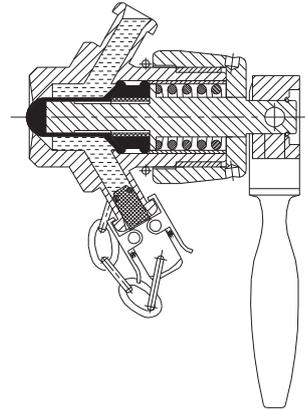
2. Remove the clip-on cap and drain the valve.
