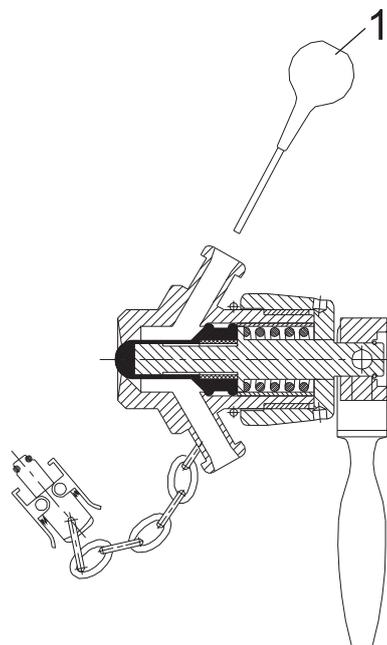
2. Put the clip-on cap on the lower connection and fill the valve with alcohol.
