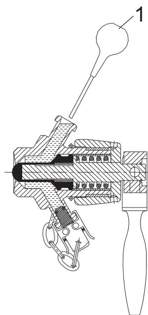
The valve is now sealed and has to be drained before the next sampling
