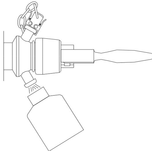
3. Close/deactivate the valve after sampling. For pneumatic valves, release the compressed air.
