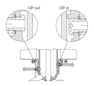
Align nozzle edges with recess in sealing element.
