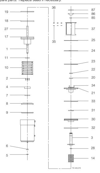
Study the instructions carefully. The items refer to the parts list and service kits section. Always use genuine Alfa Laval spare parts. Replace seals if necessary. Lubricate the rubber seals before fitting them.
