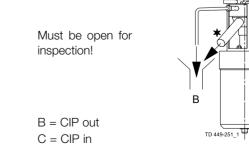
Study the instructions carefully and pay special attention to the warnings! The valve has ends for welding as standard. Weld carefully/aim at stressless welding to avoid deformation on sealing areas. Check the valve for smooth operation after welding.
