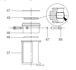
Lightly lubricate inner grove with Alfa Laval Lubricant
