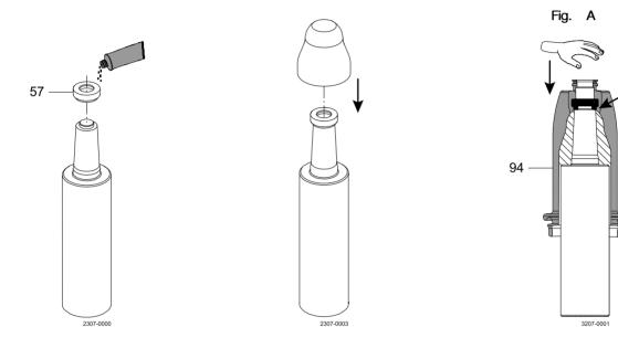
Press tank plug (93) rapidly into balanced plug (94) through the lip seal. NOTE:
