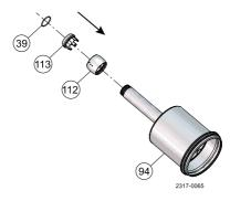
**Step 3**Nozzle and lock ring slides over spindle.
