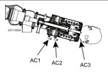
AC1 = Air connection 1 (red) upper seat push AC2 = Air connection 2 (blue) open/close AC3 = Air connection 3 (yellow) lower seat push Study the instructions carefully and pay special attention to the warnings! The valve has ends for welding as standard.
