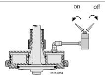
Inspect the seal to ensure it does not twist in the groove, and press in the 4 outsticking points with a screwdriver.
