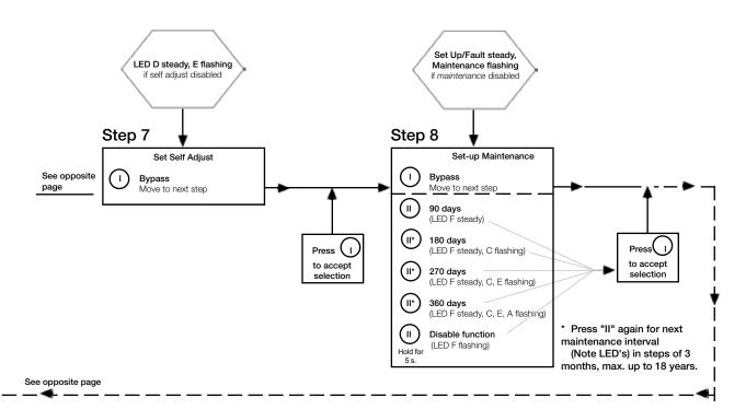
Below is stated the meaning of the LEDs' indications for fault finding in connection with the operation of the *Think*Top<sup>®</sup>.
