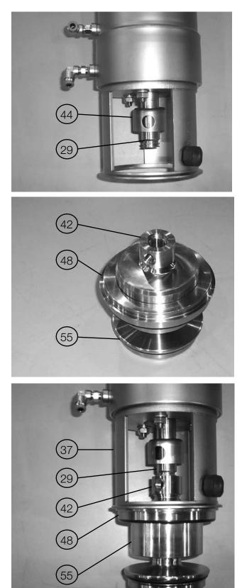
10. Install lock (44) onto piston rod (29).
