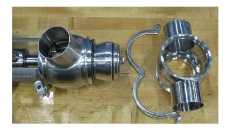
6. Remove flushing pipe using 19mm wrench.
