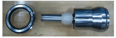
6. Ensure sealing element is orientated so the white guide ring is upwards.
