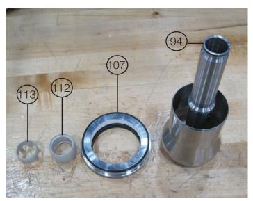
14. Remove valve body sealing element.
