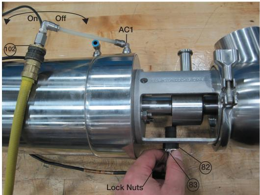
The following instructions should be made while the valve is hot from CIP cleaning. (worst case)
