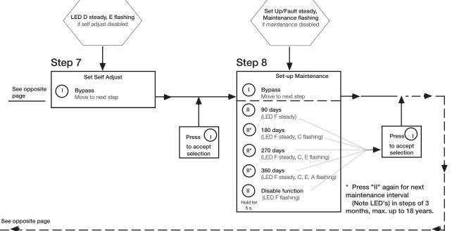
Below is stated the meaning of the LEDs' indications for fault finding in connection with the operation of the *Think*Top®.
