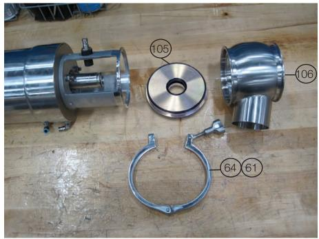
16. Remove clamp, vent body and sealing element.
