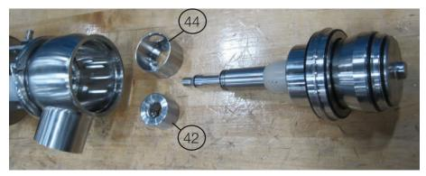
10. Turn out lower plug by hand and remove plug assembly.
