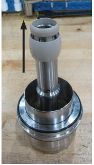
13. Remove lock ring and rotaing nozzle by pulling upwards.
