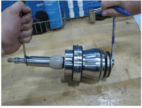
12. Remove upper stem by using a 13mm and a 16mm wrench.
