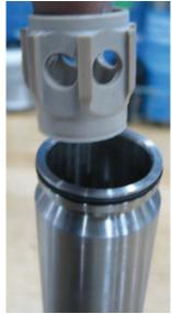
8. Insert nozzle, ensure that it is inserted as shown on picture.
