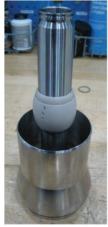
4. Nozzle and lock ring slides over spindle.
