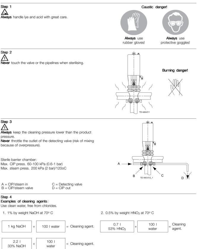
The valve is designed for cleaning in place (CIP). CIP = Cleaning In Place. Study the instructions carefully and pay special attention to the warnings! NaOH = Caustic Soda. HNO3 = Nitric acid.
