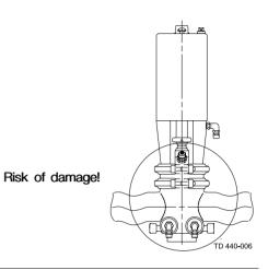
Step 4 Fittings: Ensure that the connections are tight.
