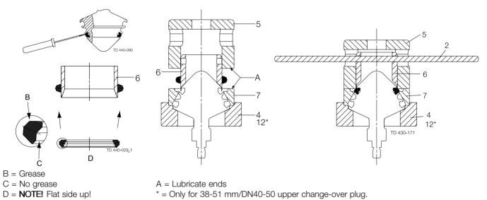
Study the instructions carefully. The items refer to the parts list and service kits - see section 7 Parts list and service kits. Handle scrap correctly. Do **not** lubricate the rubber seals or the tool parts before fitting the seals.
