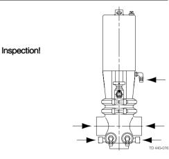
Study the instructions carefully and pay special attention to the warnings! The valve has welding ends as standard but can also be supplied with fittings. CIP = Cleaning In Place (see section 4.3 Recommended cleaning).
