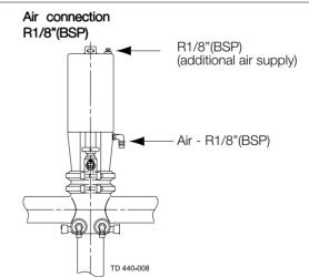
Study the instructions carefully and pay special attention to the warnings! The valve has welding ends as standard but can also be supplied with fittings. CIP = Cleaning In Place (see section 4.3 Recommended cleaning).
