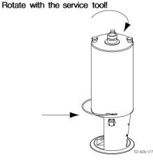
Study the instructions carefully. The items refer to the parts list and service kits - see section 7 Parts list and service kits. Handle scrap correctly. Do **not** lubricate the rubber seals or the tool parts before fitting the seals.
