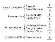
S-interface 31/62 node Sensor board Terminal strip
