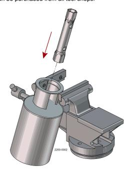
Step 3 Introduction - Aligning spindle
