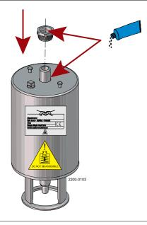
Step 7 Fit the aligning spindle to the actuator spindle, and then mount the socket wrench.
