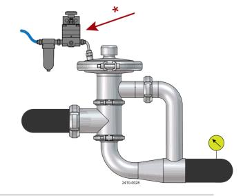
Study the instructions carefully. The valve has welding ends as standard. Weld carefully.
