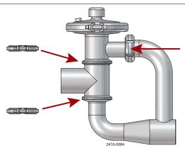
Step 13 Pre-use check: Lift and lower the valve top a few times to ensure that the valve operates smoothly. Pay special attention to the warning!
