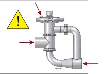
Study the instructions carefully and pay special attention to the warnings! The valve has welding ends as standard but can also be supplied with fittings. The required product pressure is preset by means of an air pressure regulating valve (optional extra).
