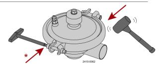
Study the instructions carefully. Lubricate the guide, the sectors and the threads before assembly. The items refer to the parts list and service kits section.
