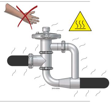
Step 3 Never touch the valve top if compressed air is supplied to the valve.
