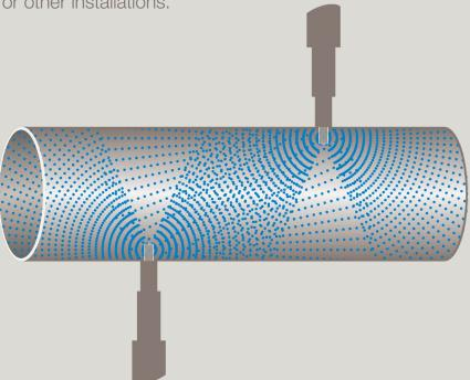
A pair of Free Rotating Retractors can provide full cleaning coverage of a large duct segment. The freely rotating spray heads remove solids, powders, and liquids inside the duct, cleaning each other in the process. After cleaning, full retraction of the spray heads prevents buildup of product inside the duct.
