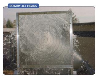
Figure 4. Impingement cleaning uses the mechanical force of the wash fluid to scour tanks clean.
