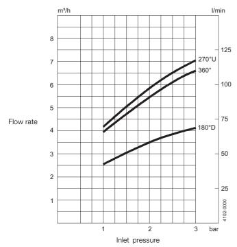
For clip-on models, the flow rate is increased by approx.  $0.5m^3/h.$
