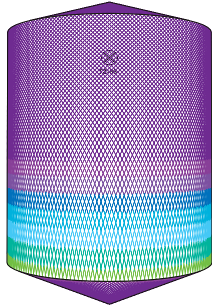
D8m H10m, Toftejorg TZ- 66, 4 x ø10 mm, 0% Tempo = 23.3 min., consumo acqua = 10868 l
